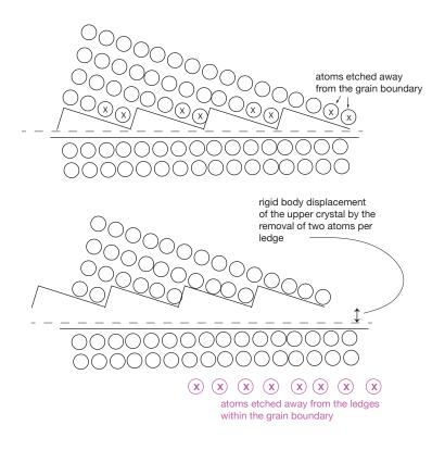
Figure 7: Etching of atoms out of the boundary at ledge sites. As a result the two crystal move closer together as rigid bodies.
