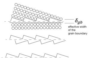
(Figure 6) Notes: (i) Any misorientation between the crystals will necessarily give rise to ledges as the boundary. (ii) The ledges may be further apart or closer in as contrasted in the bottom two drawings. (iii) In the top picture one crystal is shown to be flat. However, a change in the plane of the boundary can introduce ledges in the bottom crystal.
