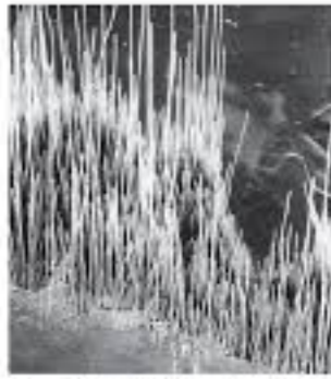
(a) Two failure modes in ceramic-ceramic composites. (b) Extensive pull-out of SiC fibers in a glass matrix provides good composite toughness. (From Metals Handbook, American Society for Metals, Vol. 8, 9th Ed., 1985) (c) Bridging of some fibers across a crack enhances the toughness of a ceramic-matrix composite. (From Journal of Metals, May 1991)
