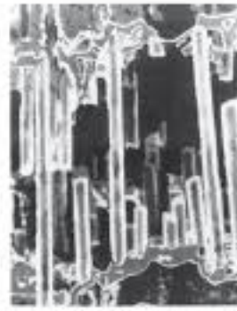
(a) Two failure modes in ceramic-ceramic composites. (b) Extensive pull-out of SiC fibers in a glass matrix provides good composite toughness. (From Metals Handbook, American Society for Metals, Vol. 8, 9th Ed., 1985) (c) Bridging of some fibers across a crack enhances the toughness of a ceramic-matrix composite. (From Journal of Metals, May 1991)
