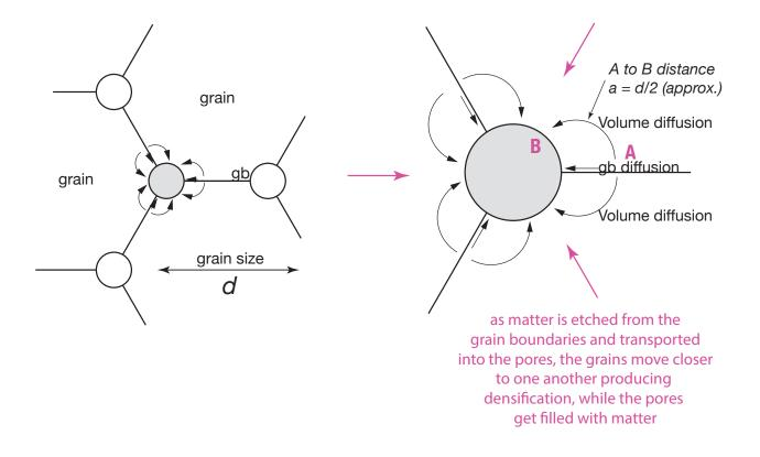
•Mass from the grain boundaries can be transported simultaneously along two paths, one through the grain matrix (volume diffusion) and the other along the grain boundary.
