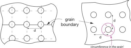
circumterence in the grain boundary plane which multiplied by the width of the grain boundary is equal to the cross section for grain boundary diffusion into the pore Let us now proceed with the above steps.
