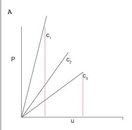
Alternatively the equations for beam flexion, which are given above can be used to simulate an experiments for silica glass. Using  $\gamma_s = 1 \, \mathrm{J} \, \mathrm{m}^{-2}$  and reasonable values for the DCB specimen calculate critical load to facture (it should be a few kg). The elastic modulus for glass is 80 GPa.
