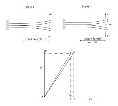
We consider two states. In the first the crack length is equal to "c" while in the second the crack is assumed to grow incrementally to " $c+\delta c$ ".
