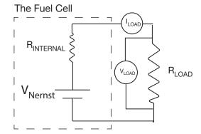
The response of a fuel cell (cell voltage and power) are shown below
