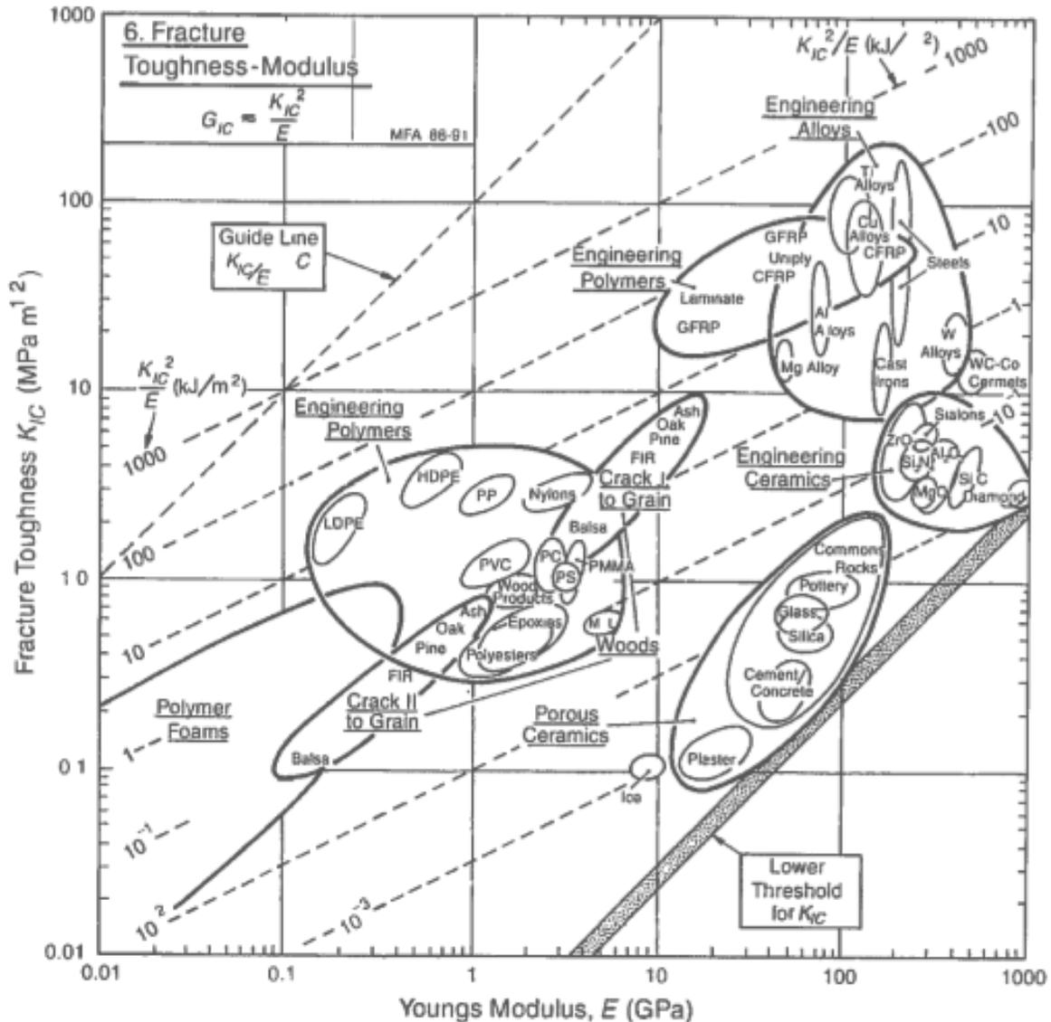
The fracture toughness for many classes of materials are shown in the map where  $K_{IC}$  is plotted against the Youngs Modulus. Once again the Youngs Modulus becomes a guide to fracture resistance. Typical range of values for different materials are:
