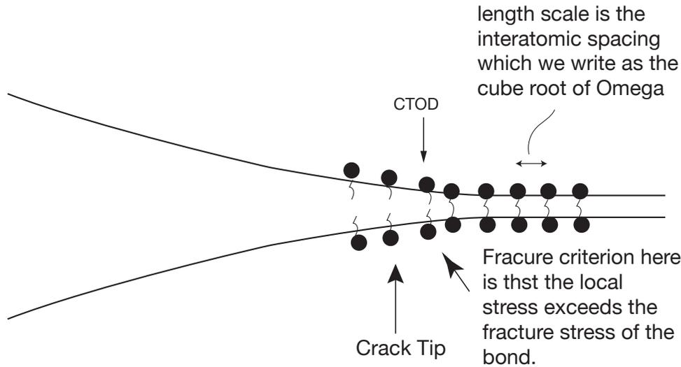
But there may be other mechanisms as well which require much more work to break the bonds. For example, in polymers the bonds are stretched until they break. This stretching of the bonds at the crack tip is shown below
