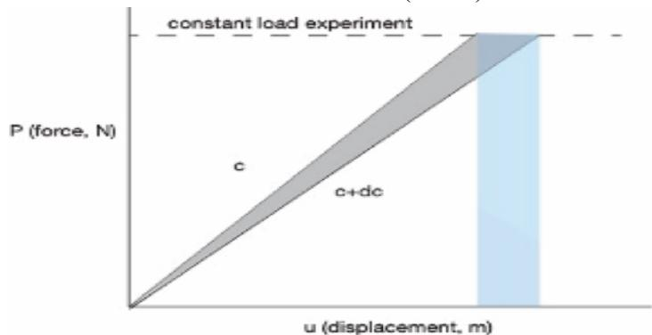
It is easy to read that the work available for fracture is greater for the low modulus material (since the area of the rectangle is greater) for the lower modulus material.
