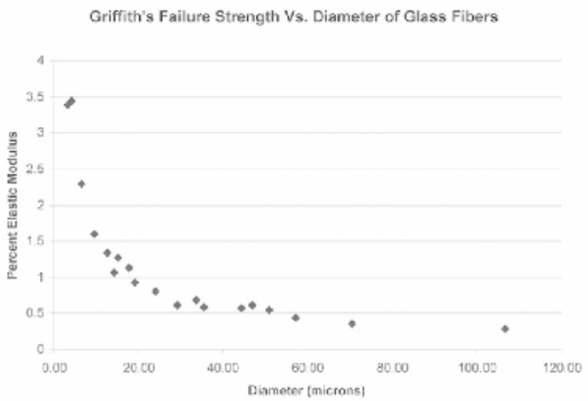
Compare the plot obtained from Eq. (1) and the experimental plot given above, converting the y-axis in the data into fracture stress expressed (assuming the elastic modulus of glass to be 80 GPa).
