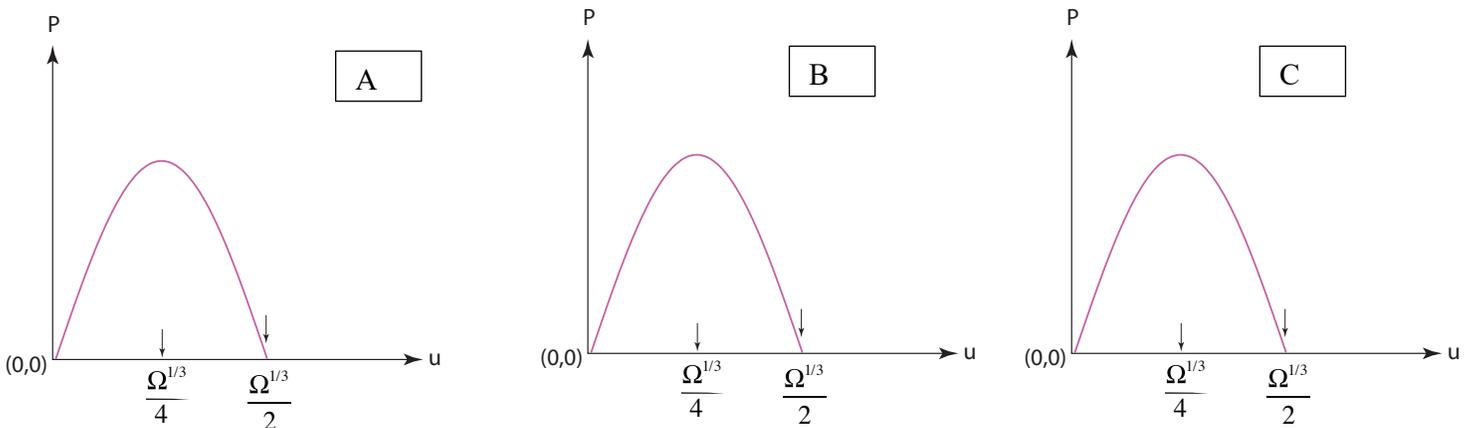
(i) Assume that material B has an elastic modulus that is 150% of A. Draw the curve for B superimposing it on the curve for A (the middle graph above).
